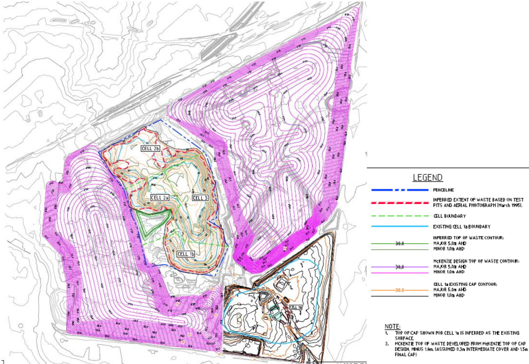
Figure 13: Pre-settlement Top of Waste Contour Plan
